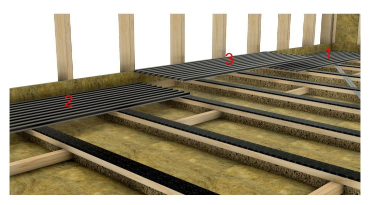
The sheets are laid alternately turned upside down. On sheet 1 and 2 the sticker is facing down, and on sheet 3 it is facing up. Then continue in the same manner with the next rows of sheets.
