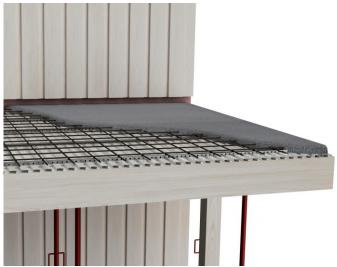
6 mm reinforcement mesh and 2.5 m free span, as well construction height of 75 mm gives a load capacity of 3.6 kN and REI 60.
