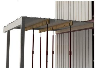
Temporary support per meter is removed only after the concrete has sufficiently hardened. Free span up to 2.5 meters
