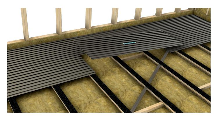
Cutting and adjustments can be made both with a jigsaw or a circular saw with hard-metal blade. If the waste is too short to be used, it is better to only shift the plates with a larger overlap.
