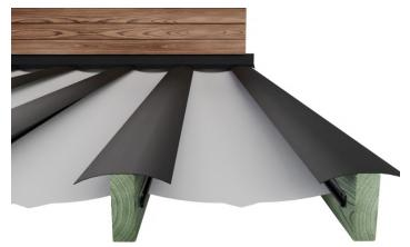
Use a 25 cm asphalt strip on top of the beams towards the wall. It is important that the strip bends down on each side of the beam.
