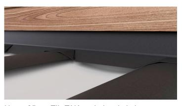
Use a 25 cm TIL-TAK asphalt strip in between wall and balcony. Make diagonal cuts in the strip as shown. It will curve downwards and the water will drain off.
