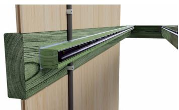
Plenty of sealant must be used between the lath and the beam, as well as around the relevant obstacle.
