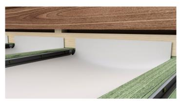
For new buildings, it is recommended to cut off more of the cord on the canvas. This way you get a larger tab that can be attached further up on the wall.
