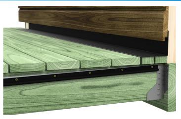
A terrace fittings are to be used towards the wall. When you retrofit, it is important to split the floorboard under the fittings! This will prevent water from being sucked towards and into the wall.
