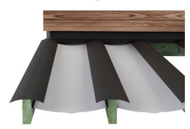
Use minimum 25 cm wide asphalt strip on top of the beams.
