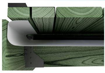
For retrofitting, fold the canvas underneath the floorboards, and it will remain in this position due to tension against the floorboards.
