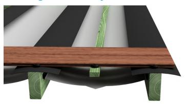
To achieve extra bracing of the floorboards you can place a lath in the center underneath, which binds all the floorboards together.
