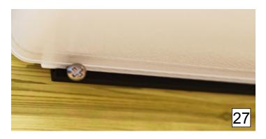
Stretching the canvas is needed. Attach a screw through the track and canvas/rope on each side close to the wall ledger.
