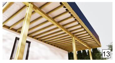
Repeat this procedure until all spaces between joists are covered.
