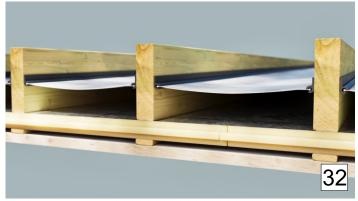
If the area under the deck is intended for enclosed spaces, e.g. conservatory or storage room; insulating underneath the joists is necessary. Polyiso insulation rigid foam boards are the only recommended insulation. These boards are moisture and fire resistant, and can be covered by soffit boards.
