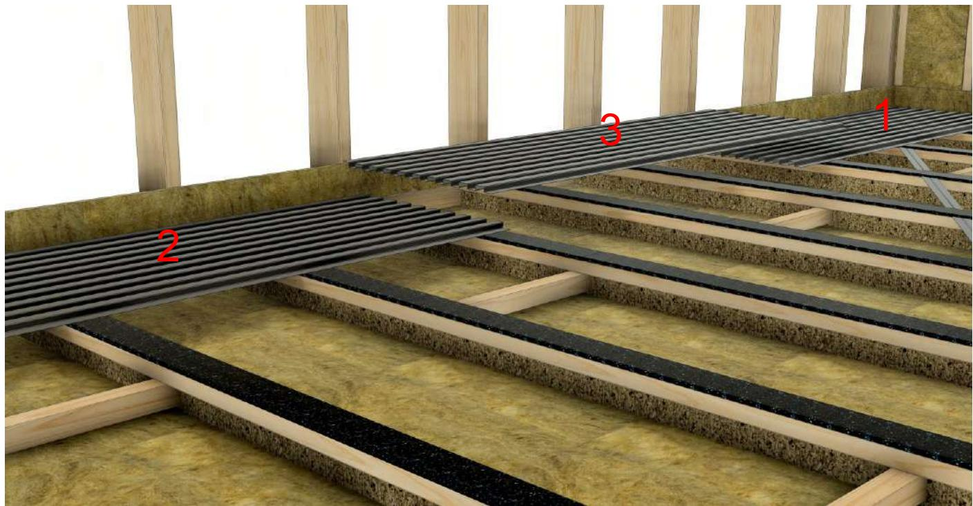
The sheets are laid alternately turned upside down. On sheet 1 and 2 the sticker is facing down, and on sheet 3 it is facing up. Then continue in the same manner with the next rows of sheets.
