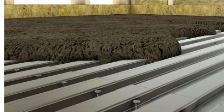
The screws / nails are placed in each corrugated bottom along all beams. The top of the screw / nail should align with the top of the sheets. Cast as described on page 4.
