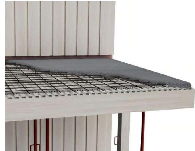
Temporary support per meter is removed only after the concrete has sufficiently hardened.
